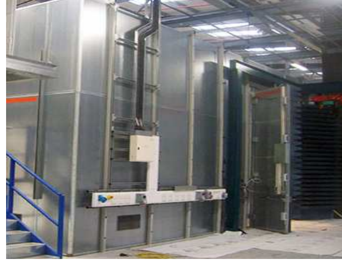
Aaronia Magnoshield® made from Mu-metal allows quick and easy large-area magnetic field screenings.
